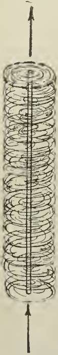
FIG. 24 Magnetic whirl surround- ing a wire through which a current is passing
